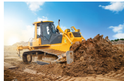
Cylinder-integrated sensors ensure optimum leveling and automated blade positioning in bulldozers
