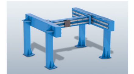
Synchronization of the feed motors for gantry drives with a separate measuring system
